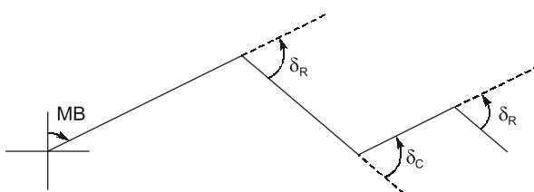
Deflection angles are the angles which a line makes with the prolongation of the proceeding line.
