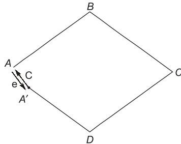
Closing error = (AA') i.e., coordinate of A' w.r.t. coordinate of A
