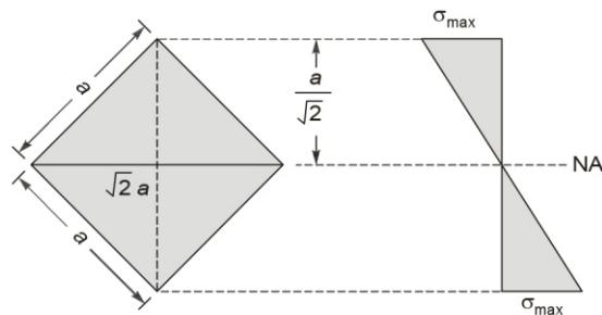
The bending stress in a beam is governed by its section modulus,
