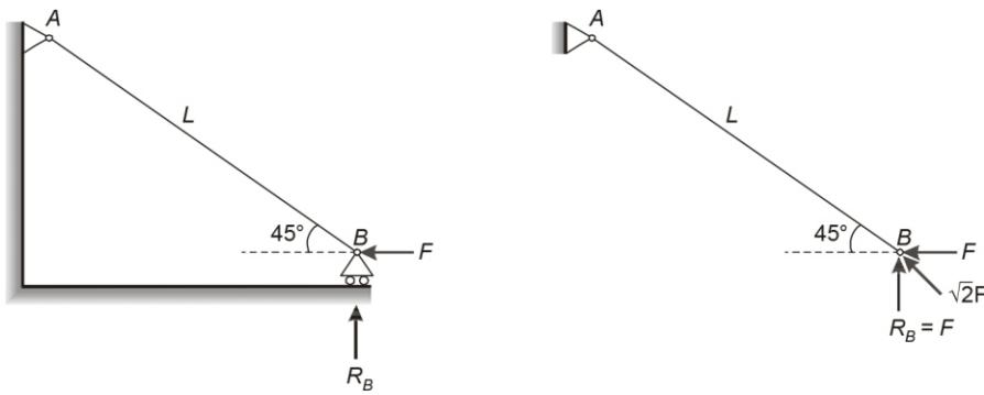
$$\begin{aligned}\therefore \sum M_A &= 0 \\ \Rightarrow R_B \times L_1 - F \times L_1 &= 0 \\ \Rightarrow R_B &= F\end{aligned}$$
