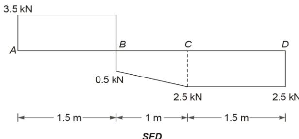
The maximum bending moment will occur at *B* because the shear force diagram changes its sign at *B*i.e., the distance of point *B* from *C* = 1 m.
