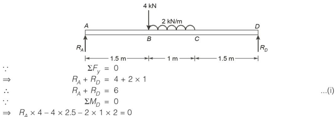
$$\Rightarrow \begin{aligned} R_A &= 3.5 \text{ kN} \\ R_D &= 6 - 3.5 = 2.5 \text{ kN} \end{aligned} \quad (\text{Using equation (i)})$$
