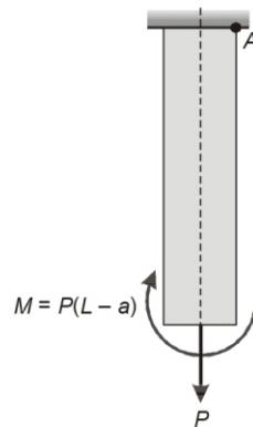
$$\text{Section modulus, } Z = \frac{2a(2a)^2}{6} = \frac{8a^3}{6}$$
