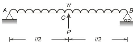
$$\text{Deflection at } C \text{ due to uniformly distributed load} = \frac{5wl^4}{384EI} (\downarrow)$$
