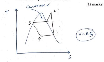
1) Liquidity the refrigerent by rejecting heat (at const P)
