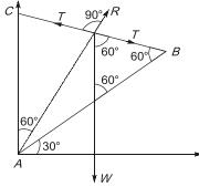
Q.12 A ladder AB of length 5 m and weight (W) = 600 N is resting against a wall. Assuming frictionless contact at the floor (B), and the wall (A), the magnitude of force P(in Newton) required to maintain equilibrium of ladder is \_\_\_\_\_.
