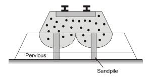
(e) **Use of capillary break**: If water pocket is created due to capillary water, a coarse grain layer is provided to cut it off.
