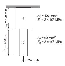
Segments 1 and 2 have cross-sectional area of 100 mm $^2$  and 60 mm $^2$ . Young's modulus of  $2 \times 10^5$  MPa and  $3 \times 10^5$  MPa, and length of 400 mm and 900 mm, respectively. Calculate the strain energy stored in the bar (in N-mm) due to the axial load
