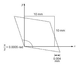
If the shear strain  $\gamma_{xy}$  at this point is expressed as 0.001 k (in rad), the value of k is
