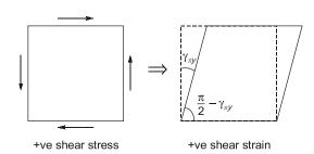
In question since angle has been increase therefore shear strain should be negative.
