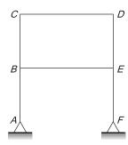
If the axial and shear deformations in different members of the frame are assumed to be negligible, then what would be the reduction in the kinematic indeterminacy.
