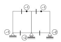
$D_s$  = 3 × Number of cuts to open-closed loops - Reaction added to make stable cantilevers
