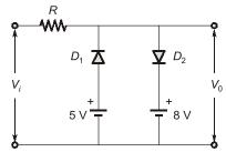
For  $V_i > 8 \text{ V} \rightarrow \text{diode } D_1 \text{ will be off and diode } D_2 \text{ will be on}$
