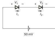
As both diodes are ideal and identical hence voltage drop across both diodes will be same.
