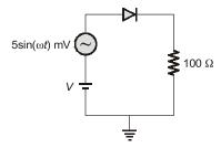
For  $\omega = 2 \times 10^6$  rad/s, the amplitude of the small-signal component of diode current.
