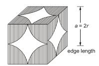
Atomic Packing Factor (APF) of the crystal structure is defined as the ratio of total volume of the atoms per unit cell to the volume of the unit cell. It is also known as packing efficiency  $(\eta)$ .
