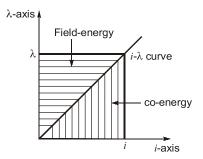
Where,  $\lambda = N\phi = \text{Flux linkage}$
