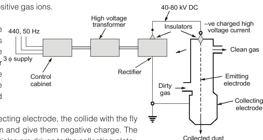
As these ions move to the collecting electrode, they collide with the fly ash particles in the gas stream and give them negative charge. The negatively charged fly ash particles are driven to the collecting plate.
