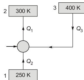
$$COP = \frac{\text{Refrigeration effect}}{\text{Work done}} = \frac{T_1}{T_2 - T_1}$$
