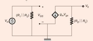
$$V_0 = -g_m V_{gs}(R_D \parallel R_L)$$
