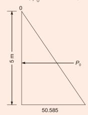
4. Total earth pressure,  $P_0 = \frac{1}{2}k_0 \cdot \gamma \cdot H^2 = \frac{1}{2} \times 0.67 \times 15.1 \times 5^2$  $= 126.46 \, kN/m$
