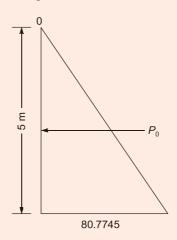
$$\gamma' = \left[ \frac{G-1}{1+e} \right] \gamma_w = \frac{2.68-1}{1+0.74} \times 9.81 = 9.47 \text{ kN/m}^3$$
