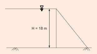
$G_c$  - Specific gravity of dam material = 2.25 Uplift factor, K = 0.45
