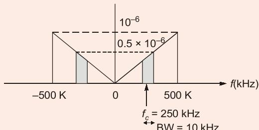
Since bandwidth of the filter is small compared to the carrier frequency  $f_c$ , we can approximate the PSD of resulting narrow band noise of  $n'(t)$  to be flat at the level of  $0.5 \times 10^{-6} \text{ W/Hz}$ .
