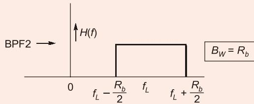
Bandwidth of bandpass filters should be equal to ' $R_b$ '
