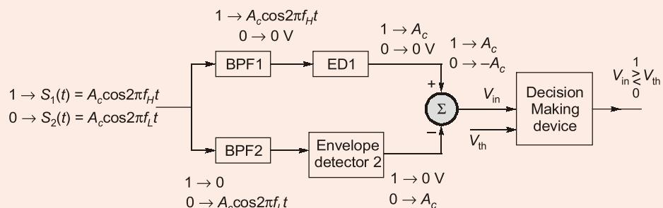
By assuming that binary sequence is represented with Nyquist pulses, band pass filters should be as follows:
