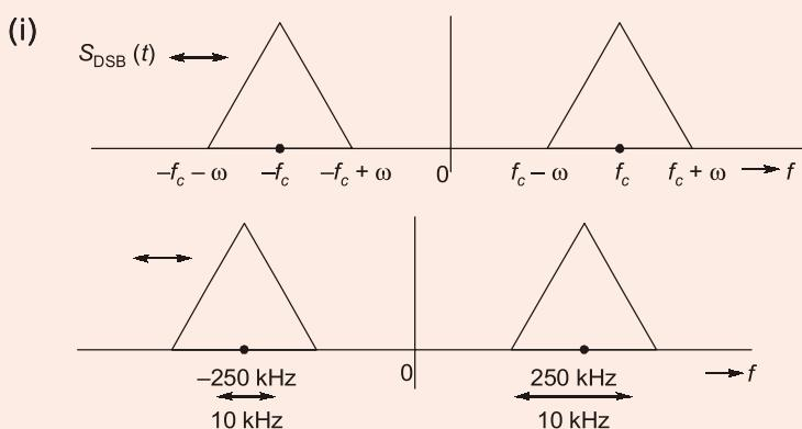
PSD of noise effecting transmitted DSB-SC signal can be obtained by passing received signal through narrow-band filter of bandwidth 10 kHz and centered about  $f_c = 250 \text{ kHz}$ .
