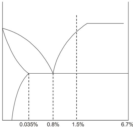
The ratio of proeutectoid cementite to total cementite is \_\_\_\_\_.
