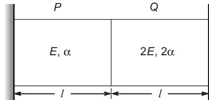
If temperature of the bar increases and  $\sigma_1 = \sigma_P$  and  $\sigma_2 = \sigma_Q$ , then
