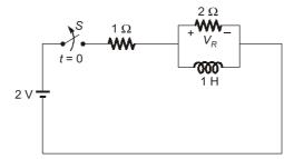
The magnitude of  $V_R$  is \_\_\_\_\_ Volts.
