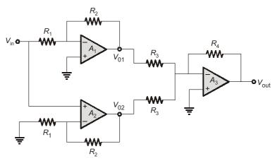
Here,  $A_1$  is an inverting amplifier and  $A_2$  is a non-inverting amplifier.
