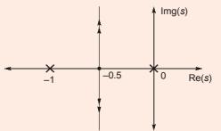
Now finding the value of K for given system having damping ratio is 0.158. The characteristic equation is 1 + GH = 0
