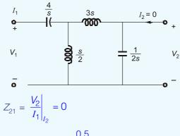
$$V_2 = \frac{I_1 \times 0.5s \times \frac{0.5}{s}}{3s + 0.5s + \frac{0.5}{s}}$$
