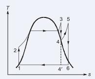
The principal advantages of reheating in Rankine cycle is to increase the quality of steam at turbine exhaust.
