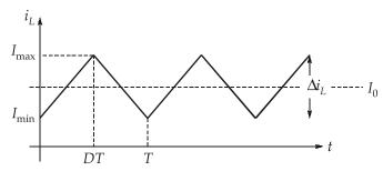
Average inductor current must be same as the average current in the load resistor.
