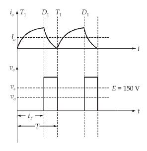
The expression for average dc machine output current is based on continuous armature inductance current. Therefore, the switching period must be shorter than the time  $t_x$ , given by below expression, for the current to reach zero, before the next switch on-period. That is  $t_x = T$  and  $\alpha = 0.30$ .
