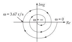
The intersection points of the plot with the negative real axis of G(s)H(s)-plane are determined using the relation given below:
