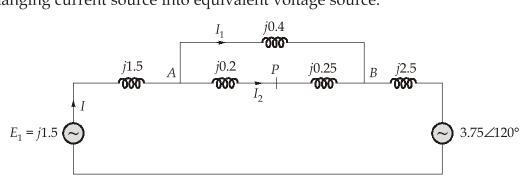
Calculate prefault voltage at point P
