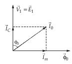
Here, no load current ( $I_0$ ) cannot lag  $\vec{V}_1$  by 90° because of core loss. In practical transformer,
