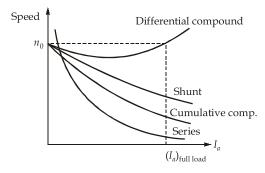
It can be seen from the characteristics, speed regulation can be zero at full load in the case of differential compound dc motor.
