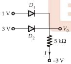
If diode  $D_1$  and  $D_2$  are made up of same material with the cut-in voltage  $V_{\gamma}$  = 0.7 V, then the value of current I is equal to
