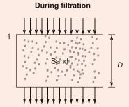
D = Depth of sand bed = 0.75 mn = Porosity of sand bed = 0.48
