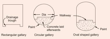
The provision of a gallery in a dam body, changes the normal pattern of stresses in the body of the dam. Stress concentration may occur at corners and hence in order to minimise this stress concentrations, the corner must be rounded smoothly. Tension and compression zones may be work out and proper reinforcement etc. are provided to counteract them.
