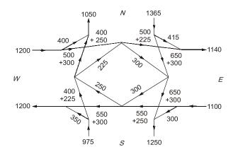
The maximum 2 way flow in the intersection leg (North) is 2415 PCU/hr and the maximum in one direction is 1365 PCU/hr.
