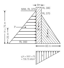
Unit weight of water =  $1000 \text{ kg/m}^3$
