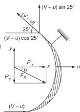
Force exerted by the jet in the direction perpendicular to direction of jet, per unit weight
