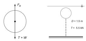
$F_{\text{buoyancy}} = \text{Tension} + \text{Weight}$
