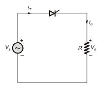
$$\begin{split} i_{T} &= i_{o} \\ \text{Form factor} &= \frac{(I_{T})_{\text{RMS}}}{(I_{T})_{\text{AVg}}} \\ &= \frac{I_{or}}{I_{o}} \\ &= \frac{V_{or} \, / R}{V_{o} \, / R} \\ &= \frac{V_{or}}{V_{o}} \end{split}$$
