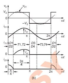
$$I_{T1} = \left[ \frac{1}{2\pi} \int_{0}^{3\pi/4} (I_{m} \sin\omega t^{2}) \cdot d(\omega t) \right]^{1/2}$$
