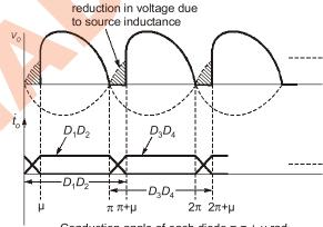
Conduction angle of each diode =  $\pi$  +  $\mu$  rad
