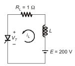
Forward voltage drop of SCR during ON-state
