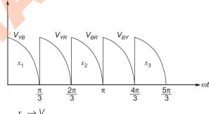
$$\begin{array}{c} x_1 \rightarrow V_{RY} \\ x_2 \rightarrow V_{YB} \\ x_3 \rightarrow V_{BR} \end{array}$$
