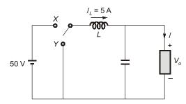
Inductor current  $i_L$  is constant and ripple free.
