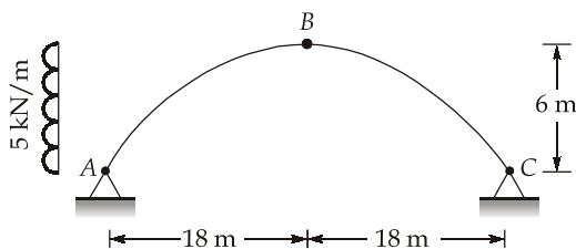
If this arch is carrying uniformly distributed horizontal load of 5 kN/m on left side, then magnitude of horizontal thrust at  $A$  is
