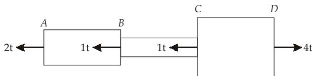
$E = 2 \times 10^6 \text{ kg/cm}^2$ . The elongation in bars are  $\Delta_1$ ,  $\Delta_2$ ,  $\Delta_3$  respectively for AB, BC and CD. The ratio of greatest to the least of these elongation will be
