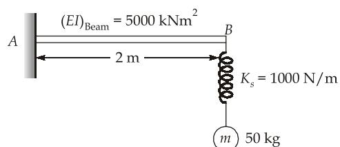
The fundamental time period of vibration of the system shown in the figure, by neglecting the self-weight of the beam, is nearly
