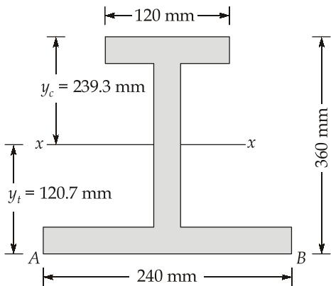
$$I_{AB} = 5.60 \times 10^8 \text{ mm}^4, \text{ Area} = 18000 \text{ mm}^2$$
