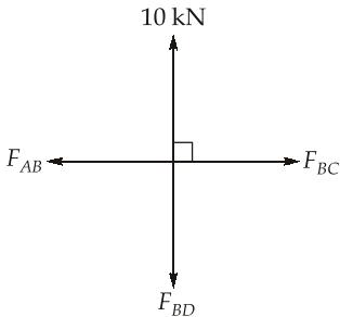
$$\begin{aligned}\therefore \text{Take } \Sigma F_x &= 0 \\ \Rightarrow F_{AB} &= F_{BC} \\ \Rightarrow F_{BC} &= \frac{40}{3} \text{ kN (T)}\end{aligned}$$
