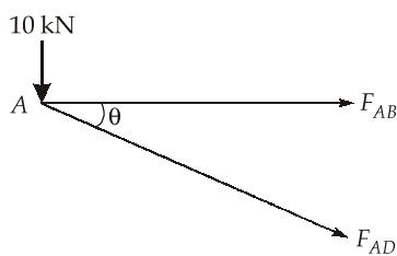
$$\begin{aligned}\Sigma F_x &= 0 \\ \Rightarrow F_{AD} \cos \theta + F_{AB} &= 0 \\ \Rightarrow F_{AB} &= -F_{AD} \cos \theta = \frac{50}{3} \times \frac{4}{5} = \frac{40}{3} \text{ kN (T)}\end{aligned}$$
