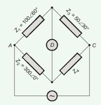
$$\begin{split} Z_1 Z_4 &= Z_2 Z_3 \\ Z_4 &= \frac{Z_2 Z_3}{Z_1} = \frac{300 \times 50 \angle 30^\circ}{100 \angle 60^\circ} \\ &= 150 \angle -30^\circ \\ &= 150 \cos 30^\circ - j150 \sin 30^\circ \\ &= R - jX_C = (130 - j75) \ \Omega \end{split}$$
