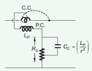
Connecting a capacitor (compensating capacitor) parallel to some part of high resistance  $(R_s)$  which is in series with potential coil.
