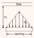
Arching action is formed and load enclosed in equilateral triangle only is fully transferred over the lintel.
