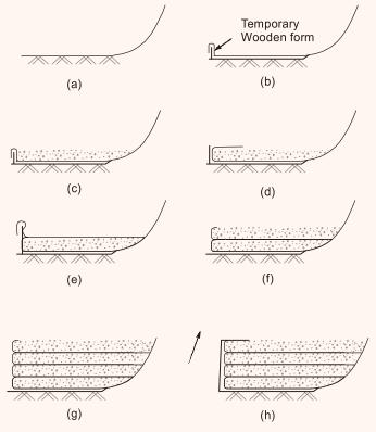
General construction procedures for using geotextiles in fabric wall construction
