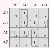
$\bar{A}\bar{C}D + \bar{A}BC + ACD + AB\bar{C}$
