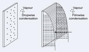
In filmwise condensation, the sliding film will act as barrier to the H.T. offering Thermal resistance between vapour and wall thereby reducing the HT rate as compared to that in dropwise condensation.
