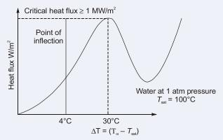
In the Nucleate boiling, beyond point of inflection, 'h' value decreases due to interference of bubbles formed on the surface of wire which will prevent the contact of liquid with wire. As such the rate of increase of heat flux with  $\Delta T$  decrease, in this region there are vapour bubbles rise as jets (OR) columns ( $\Delta T \simeq 10^{\circ}$  to 30°C) and subsequently merge into slugs of vapour.
