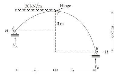
Let  $l_1$  = horizontal distance between A and C and  $l_2$  = horizontal distance between B and C
