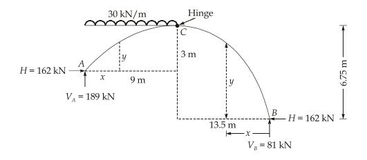
The BM at a section in AC distant x from A is given by
