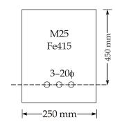
$$x_{u,\text{lim}} = 0.48d = 0.48 \times 450 = 216 \text{ mm}$$
