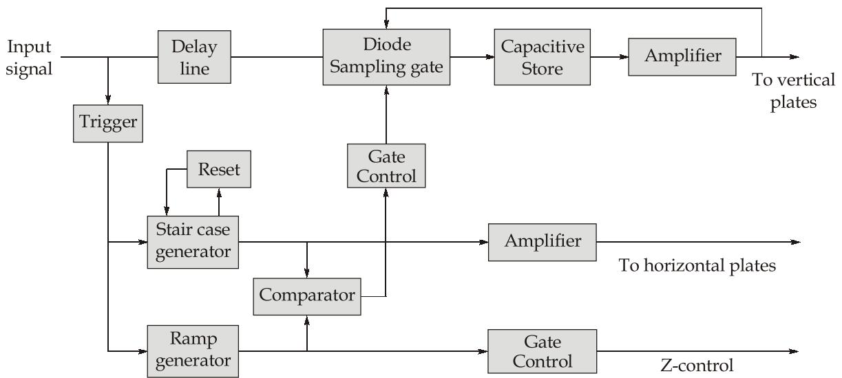
The staircase is reset after a certain number of steps, typically 100 to 1000 points are used to create the waveform on the screen.
