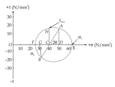
The principal stresses and their directions can be obtained from a scaled drawing, but we shall calculate  $\sigma_1$ ,  $\sigma_2$  and others values.
