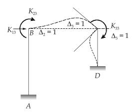
To generate the third column of the stiffness matrix, give a unit displacement at coordinate 3 as shown below. The forces required at the coordinates are:
