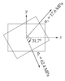
Maximum shear stress =  $\tau_{\text{max}}$  = CH = AC = 22.36 MPa
