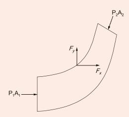
$F_x$  and  $F_y$  = Force exerted by bend on water in x and y direction
