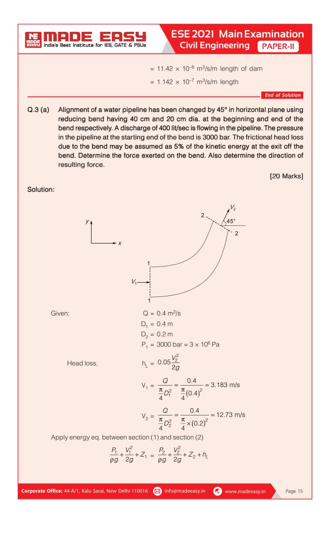
ESE 2021 Main Examination Civil Engineering PAPER-II  $(Z_1 = Z_2)$   $\frac{P_1}{\rho g} + \frac{V_1^2}{2g} = \frac{P_2}{\rho g} + \frac{V_2^2}{2g} + 0.05\frac{V_2^2}{2g}$
