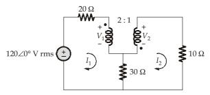
$$V_1 = -2V_2;$$
