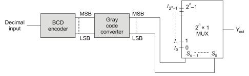
If the decimal input is 92 then  $Y_{\text{out}}$  corresponds to  $I_m$ , then value of m is \_\_\_\_
