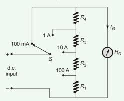
What are the values of resistances  $R_1$  ,  $R_2$  ,  $R_3$  and  $R_4$ , if the shunt resistances are connected as shown in the figure?
