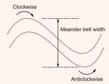
The distance between outer banks of two adjacent clockwise an anticlockwise meanders is known as meander belt width.
