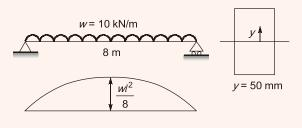
$$\sigma = \frac{M_{\text{max}}Y}{1} = \frac{\left(\frac{10 \times 8^2}{8}\right) \times 10^6}{10 \times 10^5} \times 50 = 4000 \text{ N/mm}^2$$
