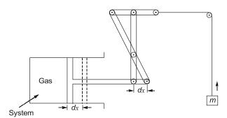
During this expansion process, the external pressure is always infinitesimally smaller than the gas pressure.
