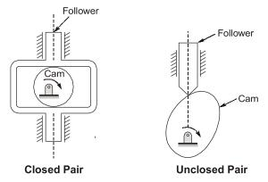
(ii) **Unclosed pair:** When two links of a pair are in contact either due to force of gravity or some spring action, they constitute an unclosed pair. In this, the links arc not held together mechanically. e.g., cam and pair shown in the figure.
