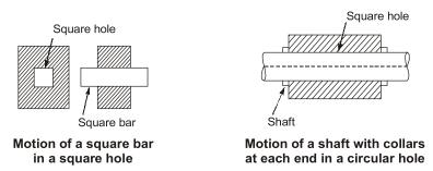
e.g. piston and cylinder (in a steam engine) form a pair. Motion of the piston is limited to a definite direction (i.e. it will only reciprocate) relative to the cylinder irrespective of the direction of motion of Round hole the crank.
