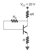
Q.13 In the given circuit ' $\beta$ ' of the transistor is 50. Assuming  $V_{CE \text{ (sat)}} = 0.2 \text{ V}$  and  $V_i = +10 \text{ V}$ , the transistor will be operating in
