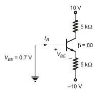
**Q.3** The collector voltage  $V_C$  of the circuit shown in the given figure is approximately
