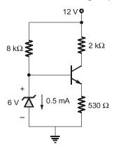
Q.12 A BJT biased in active region with B-E junction forward biased  $V_{BF} = 0.7$  V. The ' $\beta$ ' of transistor to
