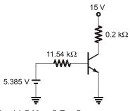
$$\begin{split} 5.385 - 11.54I_B - 0.7 &= 0 \\ I_B &= 0.406 \, \text{mA} \\ I_C &= \beta I_B = 20.29 \, \text{mA} \\ 15 - 2 \times 20.29 &= V_{CE} \\ V_{CE} &= 10.942 > V_{CE \, \text{sat}} \end{split}$$
