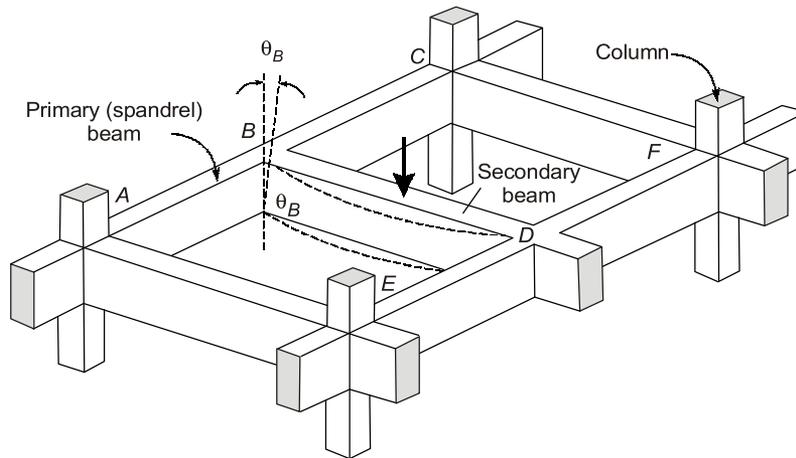
**Fig.** Concept of Compatibility Torsion
