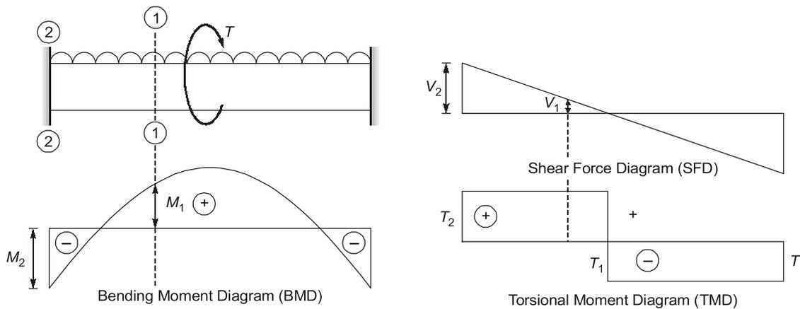
Fig. Variation of BM, SF and TM diagram in a fixed beam
