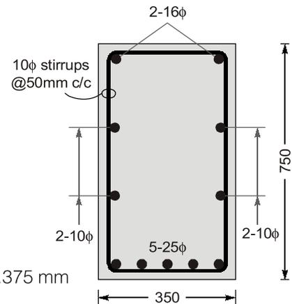
Provide 2 legged 10 mm diameter bars as shear stirrups @ 50 mm c/c.
