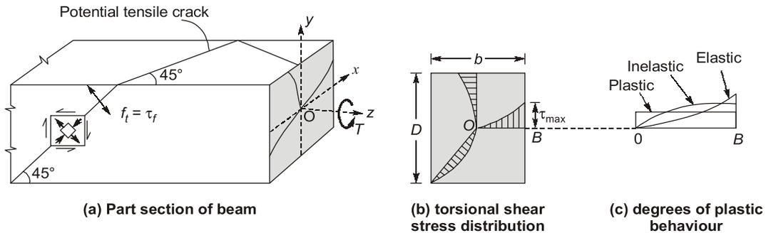
**Fig.** Distribution of Torsional Shear Stress in Elastic Rectangular Beam Section
