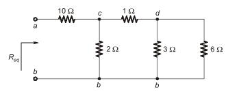
Further 3  $\Omega$  and 6  $\Omega$  in parallel gives equivalent resistance =  $\frac{3 \Omega \times 6 \Omega}{(3+6) \Omega} = 2 \Omega$
