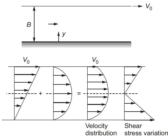
$$u = \frac{V_0 y}{B} + \frac{1}{2\mu} \left( -\frac{dP}{dx} \right) (By - y^2)$$
