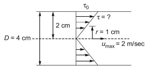
$$\therefore \tau_0 = \frac{8\mu\bar{u}}{D} = \frac{8 \times 1.6 \times 10^{-3} \times 1}{4 \times 10^{-2}} = 0.32 \text{ N/m}^2$$
