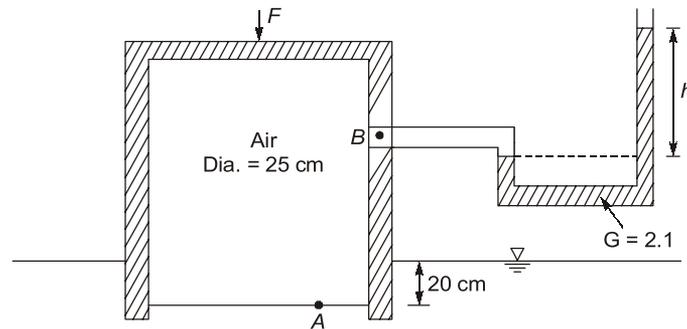
Determine the differential height 'h' of the manometer and the force 'F' Needed to hold the container at position shown in figure.
