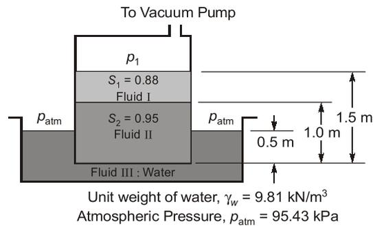
Estimate the gauge pressure value (in  $\text{kN/m}^2$ , up to two decimal places) of  $p_1$ .
