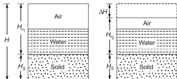
**Fig. Settling compaction**
