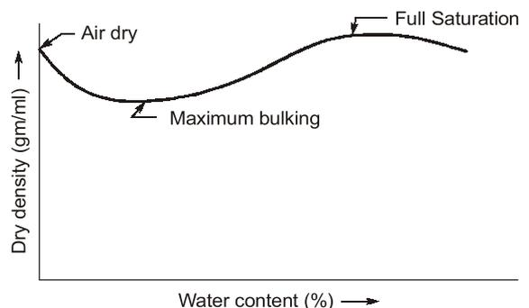
**Fig.** Compaction Behaviour of Sand
