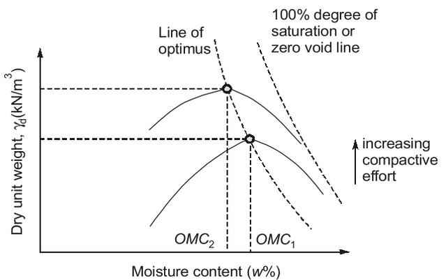
Fig. Compaction Curve
